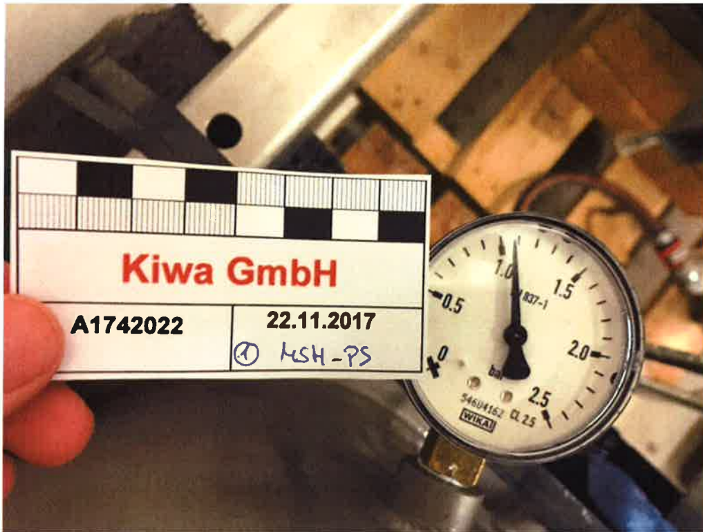
Figure A1. Water tightness test with \geq 1,0 bar water filled test cylinder (manometer at the beginning of testing on 22.11.2017).
